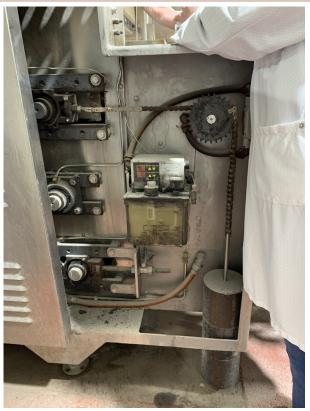
Bill Spitzer & Associates was called to inspect a malfunctioning tortilla oven chain lubrication system. We arrived on-site to provide a free of charge site investigation report and designed 4 lubrication system solutions. These systems had varied plans and installation requirements for the customer to determine which would meet operational and budgetary needs. After option 1 was selected, Bill Spitzer & Associates installed and commissioned the lubrication system ahead of time and under budget.
